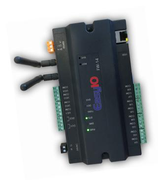
The FW (WiFi) series supports IT network and security standards and WiFi b/g/n. This series can be used as part of an existing network or as an isolated BMS WiFi network. The dual Ethernet port capability allows for daisy chain capability within the recommended IT standards.
